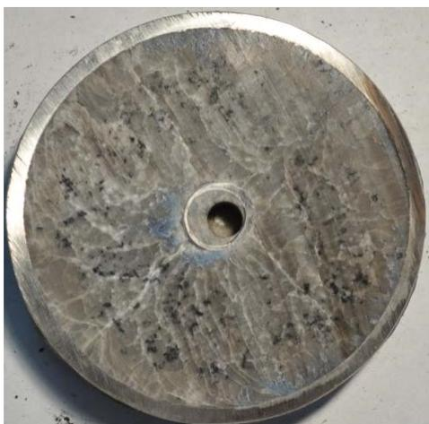
**Figure 5-4. Graphite Particle Dispersion Within Frozen Flinak in a Crucible Containing 316L, Graphite, and Metallic Sodium Held for 1,000 Hours at 850°C**
