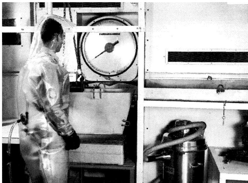
**Figure 6-5. An MSRE Employee Measuring Quantities of Salt for Production of Flibe**
