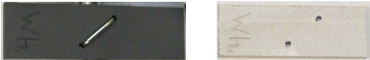
**Figure 5-2. Typical Graphite Coupon Appearance Before Exposure to Flinak at 850°C for 1,000 hours (left) and After Cleaning Showing the Presence of the Chrome Carbide Coating (right)**
