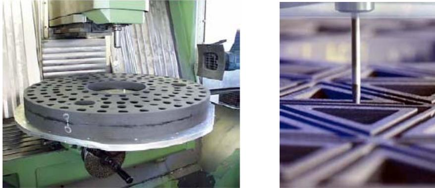
**Fig. 6** Photos of numerically-controlled milling being performed on carbon-carbon green-body material [5].
