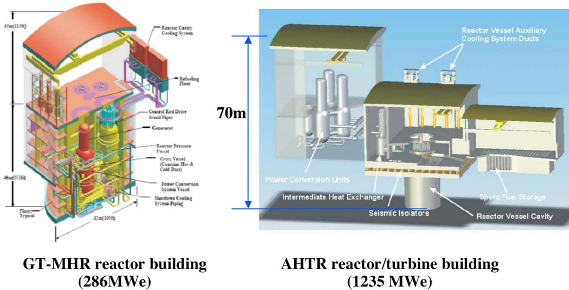
**Fig. 4** GT-MHR and AHTR reactor buildings comparison (to scale) [7, 8]
