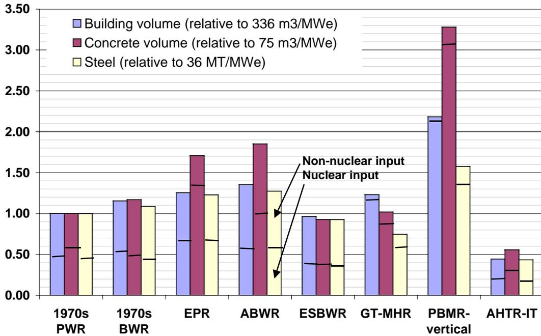
**Fig. 5** Comparison of building volume, concrete input, and total steel input for several nuclear power plants
