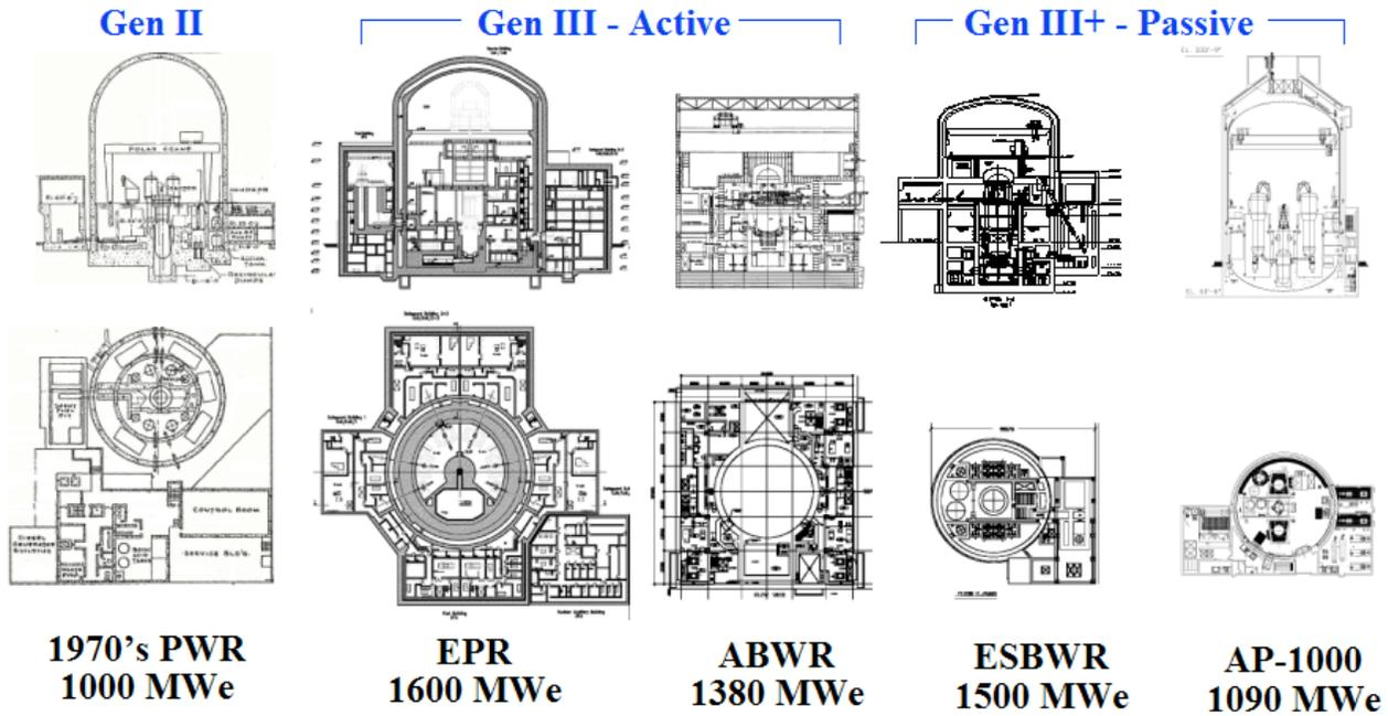
**Fig. 2** Scaled comparison of plan and elevation drawings of the reference LWRs, with rated powers ranging from 1000 to 1600 MWe
