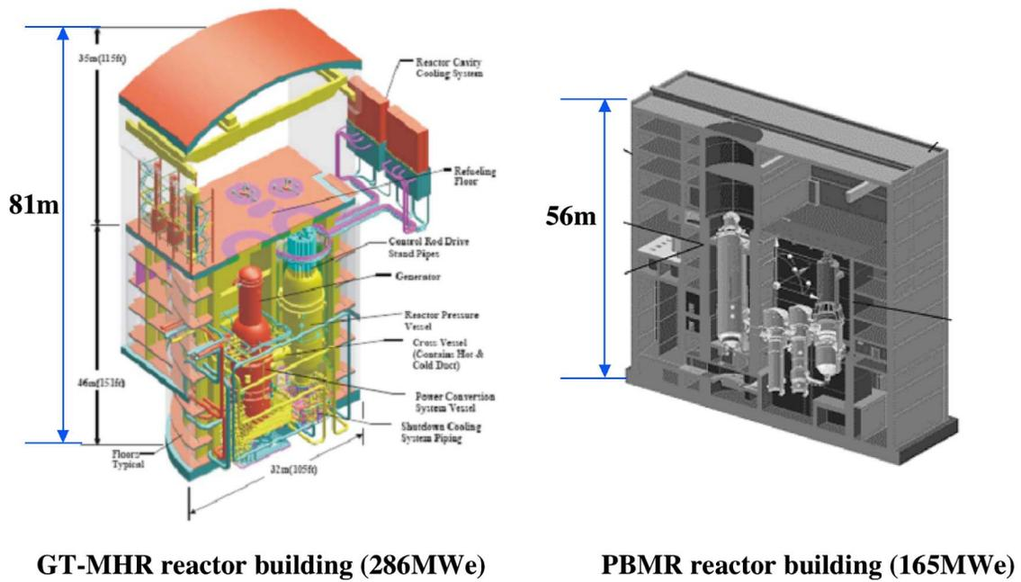
**Fig. 3** GT-MHR and PBMR reactor buildings (to scale) [7, 10]
