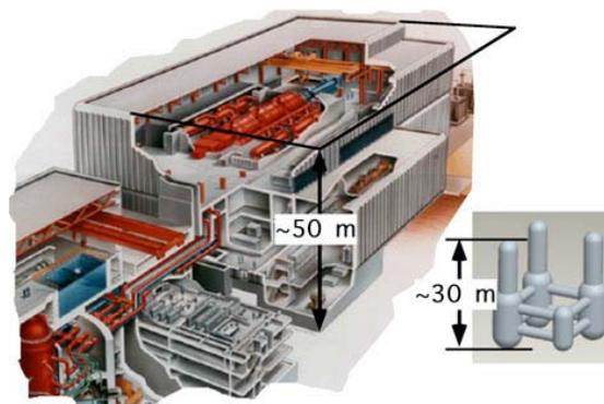
**Fig. 6.** Size comparison between the power conversion units of an intermediate-high-temperature, 1245 MW(e) MCGC-IT, and the 1380 MW(e) turbine building of the Advanced Boiling Water Reactor.
