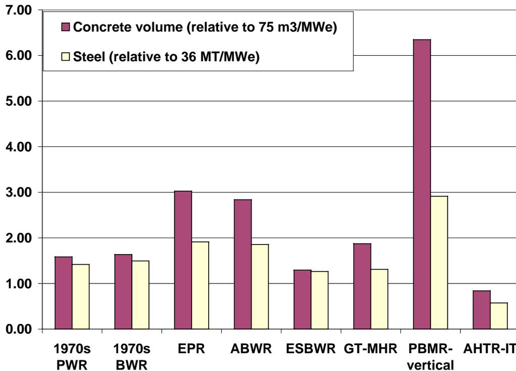
**Fig. 7** Total equivalent specific concrete and steel input (nuclear input times 2 + non-nuclear input) for several nuclear plants.
