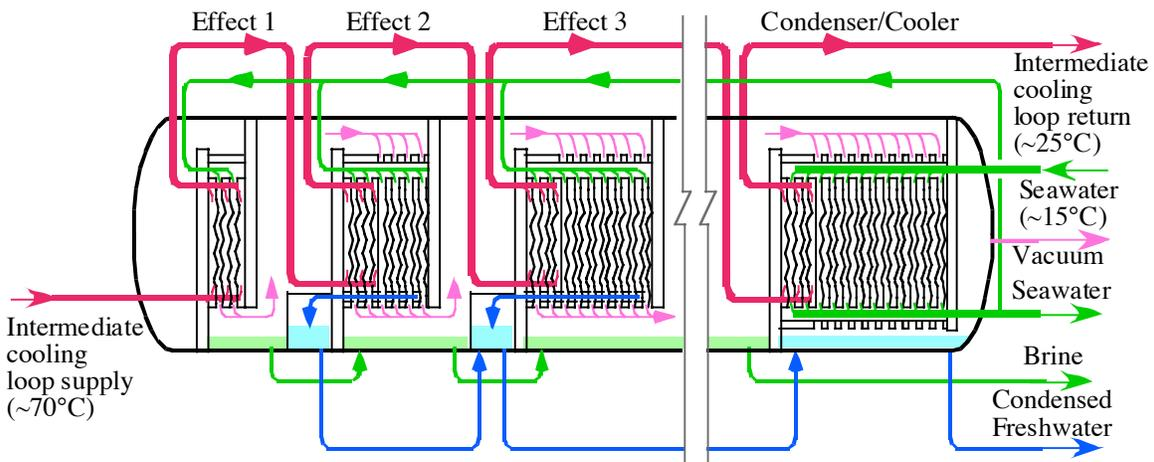
**Fig. 8** Schematic diagram of flow inside a plate-type AMED system..
