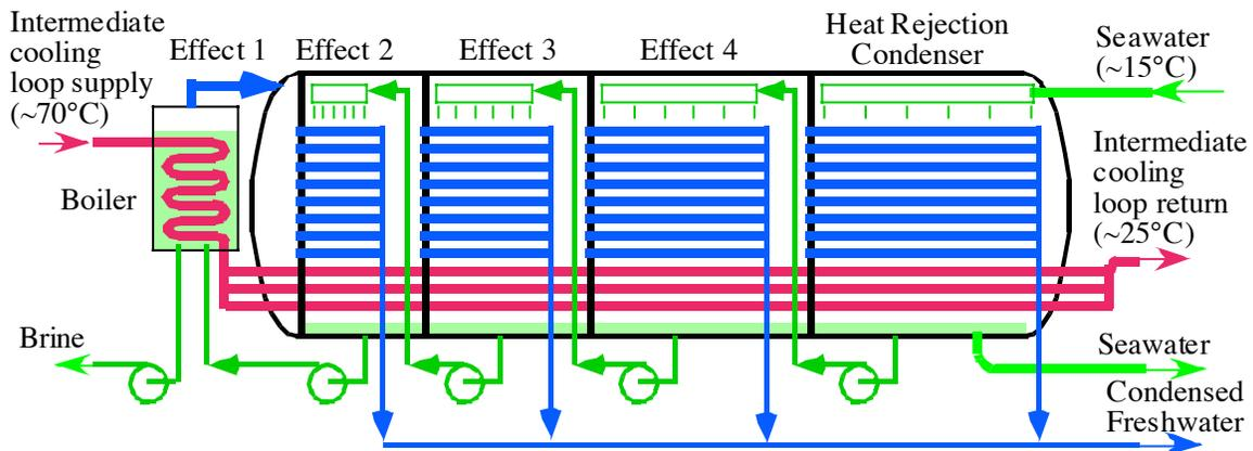
**Fig. 3** Schematic of an AMED system with four effects stages and counter-current brine flow.
