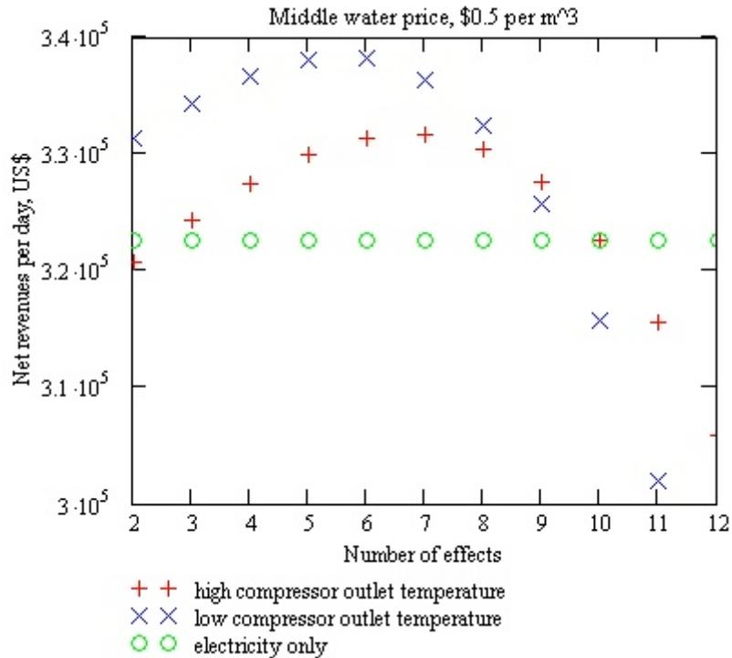
**Fig. 17** Net revenues per day for a combined power and AMED desalination plant for a water price of \$0.50/m<sup>3</sup>.
