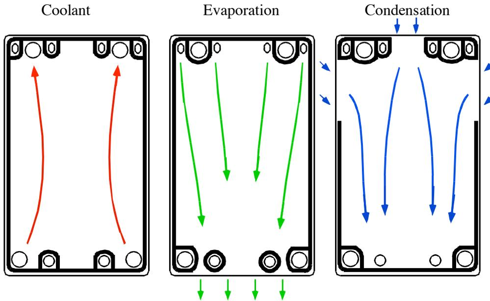
**Fig. 9** Schematic gasket configurations for AMED with plate-type heat exchangers.
