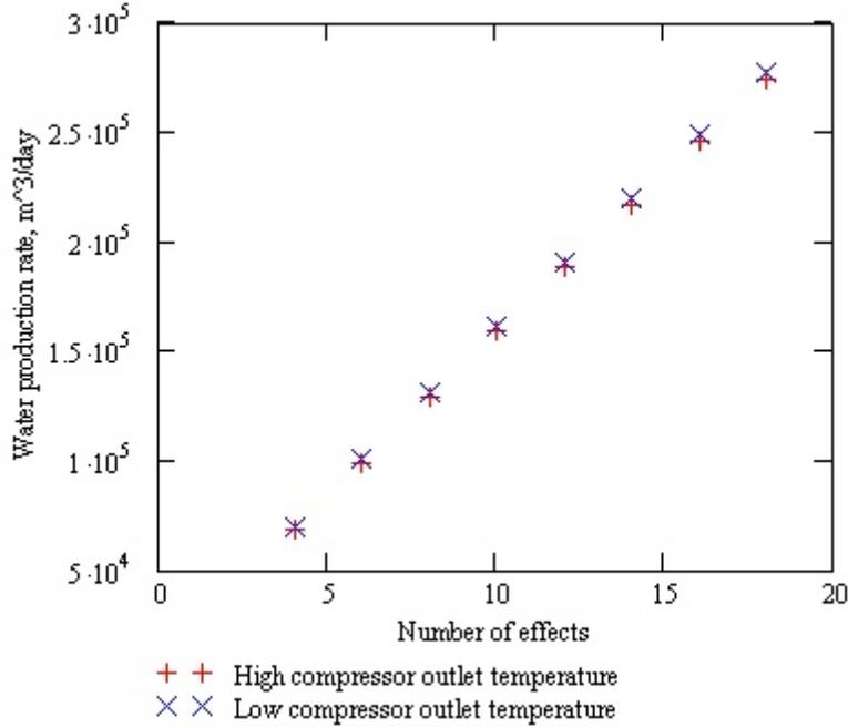
**Fig. 14** Water production rate for a 2400 MW(t) HTR as a function of number of AMED effects.
