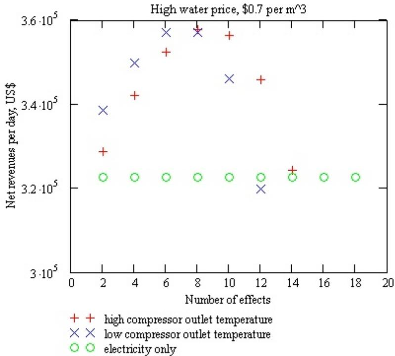
**Fig. 16** Net revenues per day for a combined power and AMED desalination plant for a water price of \$0.70/m<sup>3</sup>.
