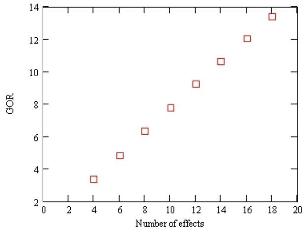
**Fig. 13** GOR for conventional MED as a function of number of effects.
