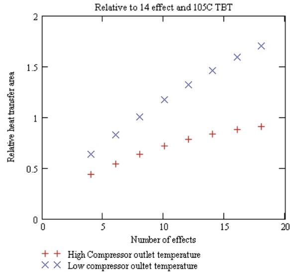
**Fig. 11** Relative specific heat transfer area per effect as the function of number of effects and TBT (142°C for HT-MED and 86°C for LT-MED).
