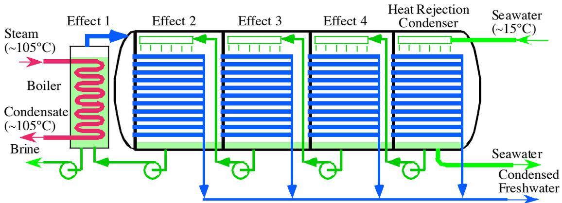
**Fig. 1** Schematic of a conventional MED system, using steam as a heat source, with four effects stages.
