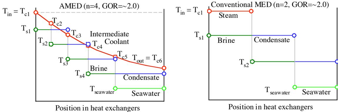
**Fig. 4** Comparisons of temperature distributions in a three-effect AMED system (Fig. 3), versus conventional MED (Fig. 1).
