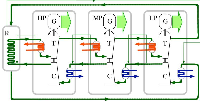
**Fig. 10** Schematic flow diagram for the reference three-expansion-stage MCGC, using three PCU modules (HP, MP, and LP) each containing a generator (G), turbine (T), compressor (C), and heater and cooler heat exchangers, with a recuperator (R) located in a fourth vessel.
