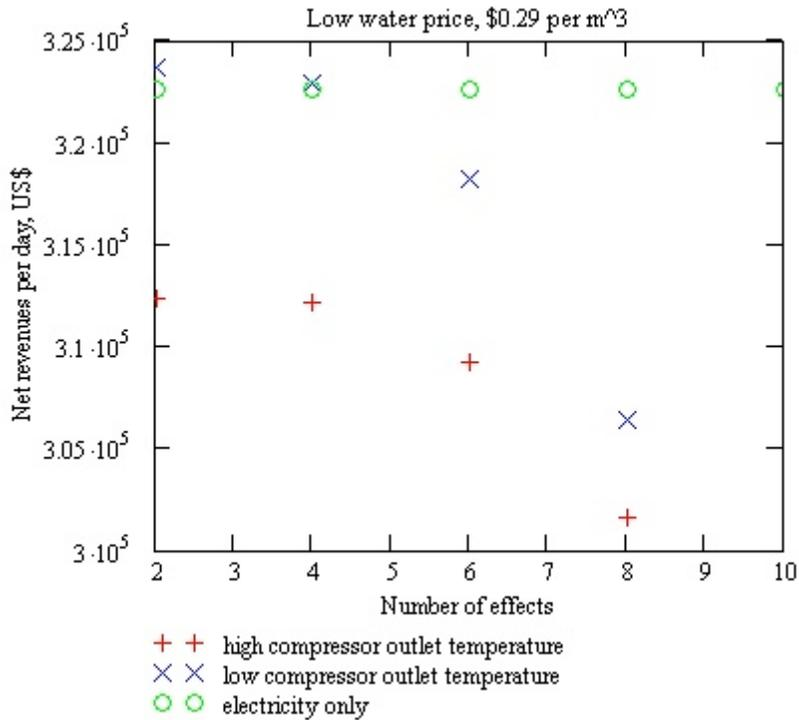
**Fig. 15** Net revenues per day for a combined power and AMED desalination plant for a water price of \$0.29/m<sup>3</sup>.
