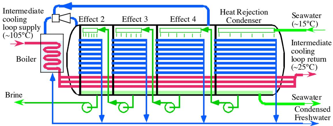
**Fig. 5** Schematic of a MED system using a single boiler and thermocompressor. Additional boilers and thermocompressors, operating at lower pressures, may be added to increase the system GOR.
