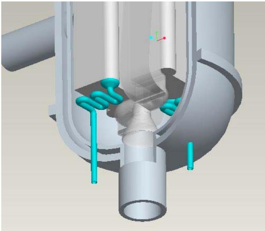
**Fig. 5** Baseline 50 MW(t) IHX design, bottom view.
