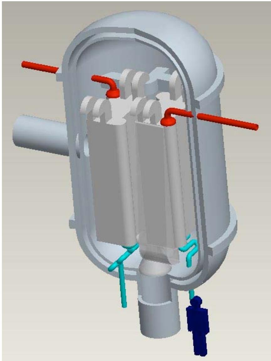
**Fig. 2** Baseline 50 MW(t) IHX design. Hot, high-pressure helium enters from the bottom and exits from the side of the IHX pressure vessel.
