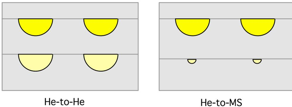
**Fig. 3** Schematic of He-to-He and He-to-MS Heatric IHX flow channels.
