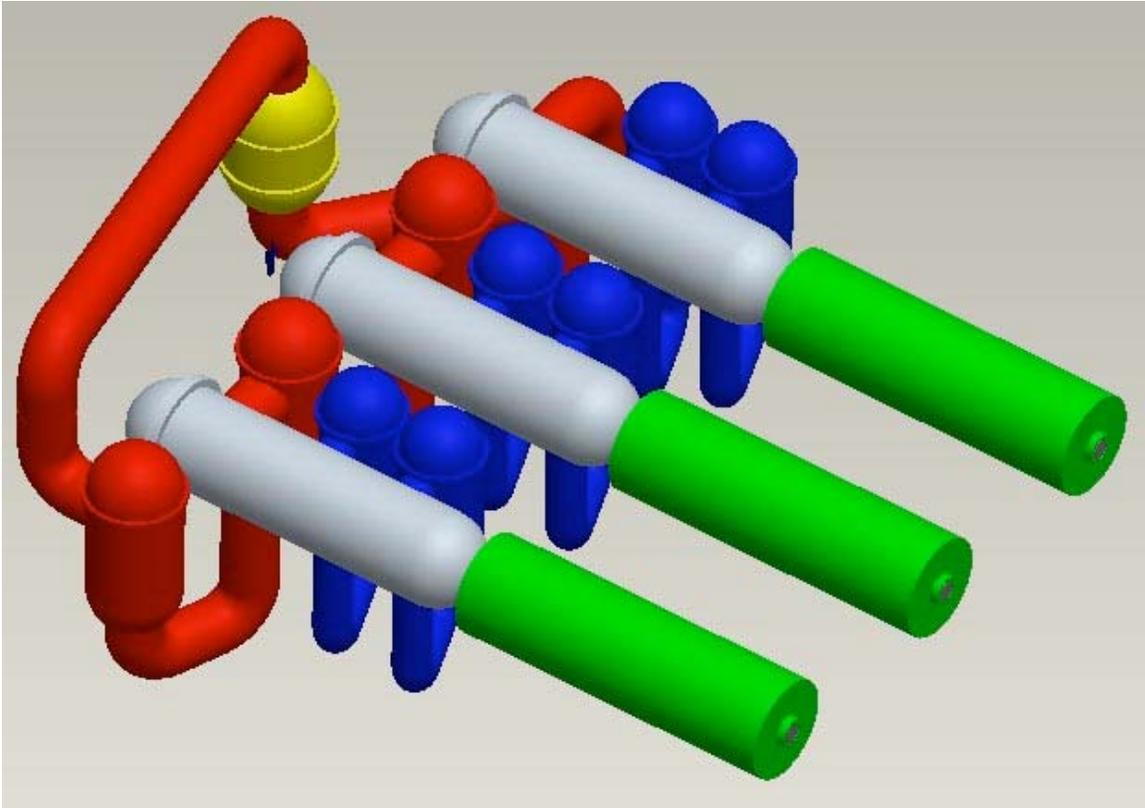
**Fig. 6** Example of a multiple-reheat gas Brayton cycle system with a distributed configuration of heaters (red), coolers (blue), recuperator (yellow) and turbomachinery (grey) [7].
