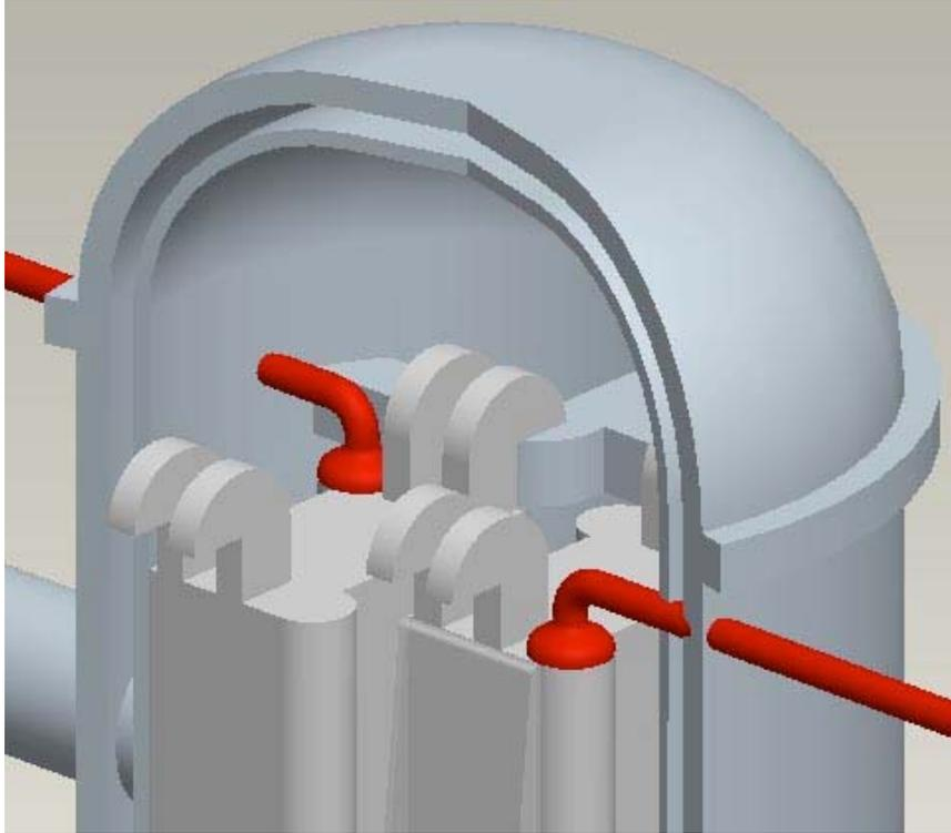
**Fig. 4** Baseline 50 MW(t) IHX design, top view.
