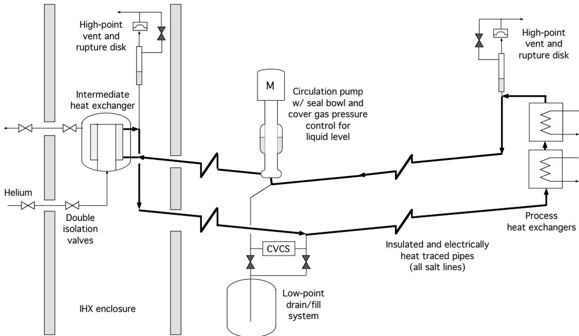
**Fig. 1** NGNP LS intermediate loop flow diagram.
