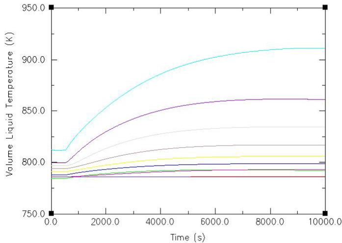
**Fig. 5** Transient response of the reference PB-AHTR buffer salt temperature, in Kelvin, at various elevations.
