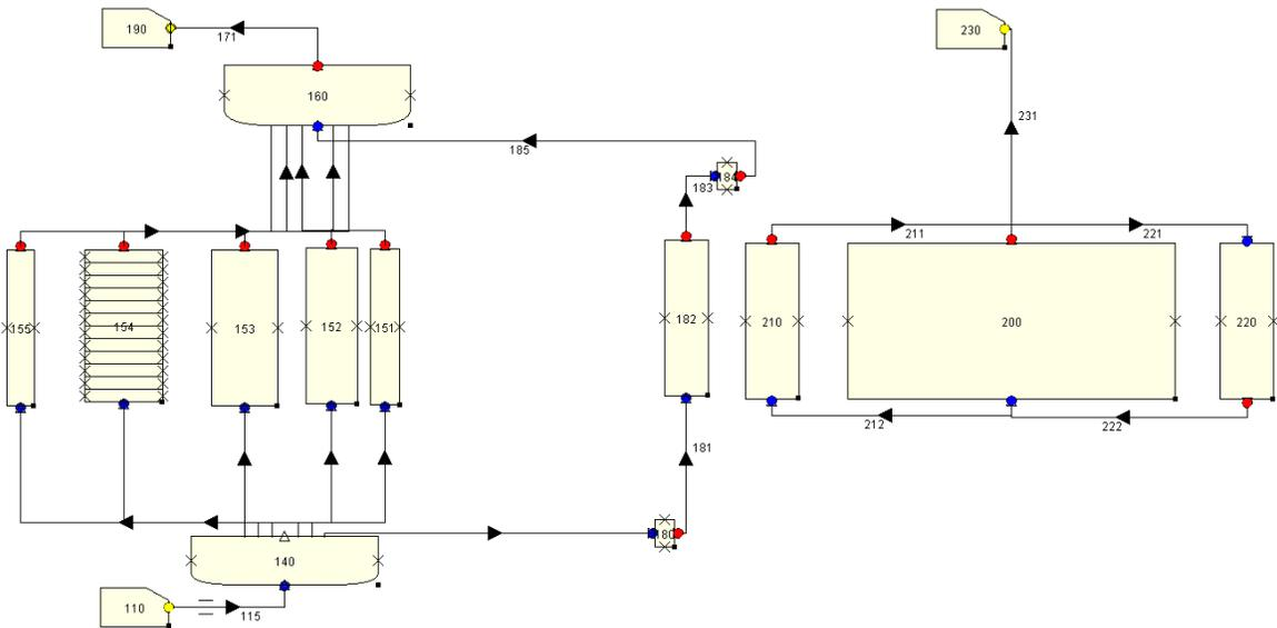
**Fig. 2** RELAP-5 nodalization for LOFC transient analysis of the PB-AHTR. (151-154: Core (different radial positions); 155: Reflector; 140-160: Plenums; 181: Fluidic diode; 182: PHX (primary side); 200: Buffer tank; 210: PHX (buffer side); 220: DHX)
