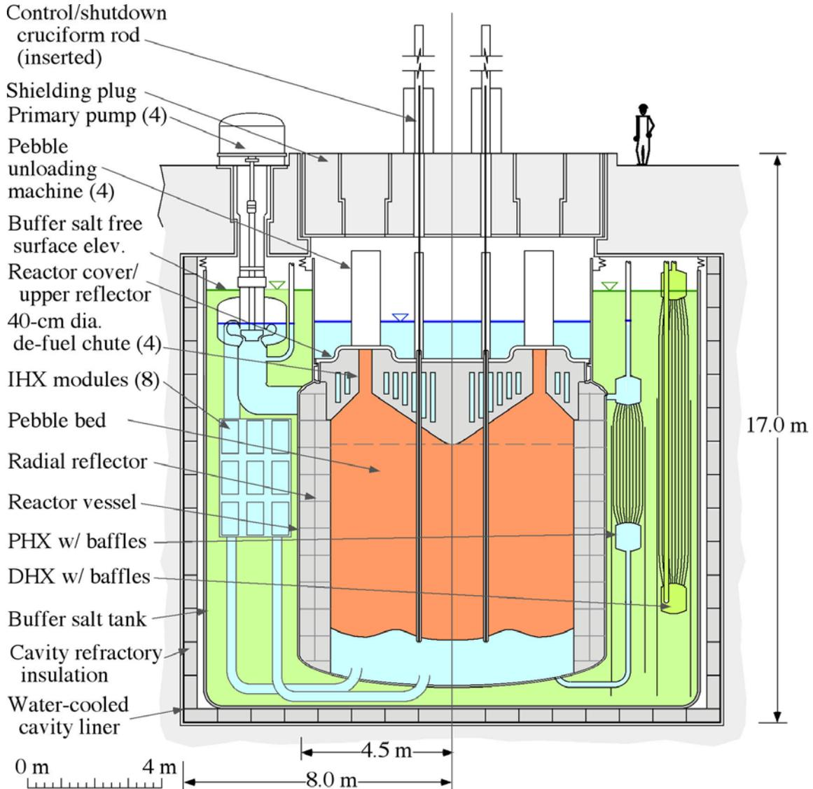
**Fig. 1** Elevation view of the PB-AHTR, showing the elevation and height of the current reference PHX design.
