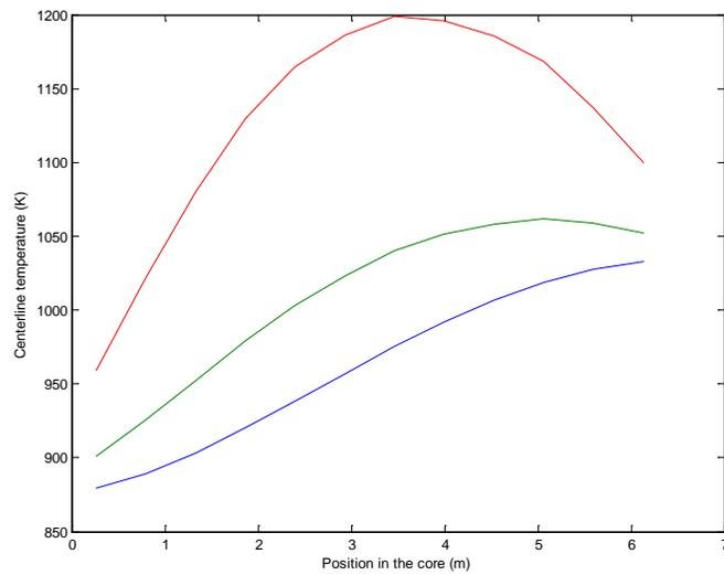
**Fig. 3** Initial steady state temperature distribution, in Kelvin, along the centerline of the PB-AHTR core, for the coolant (blue), pebble surface (green) and pebble centers (red).
