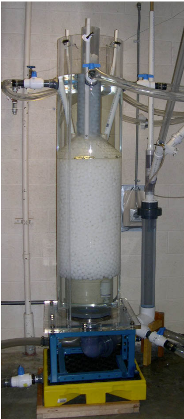
Figure 3-2: View of PREX, fully loaded with pebbles.
