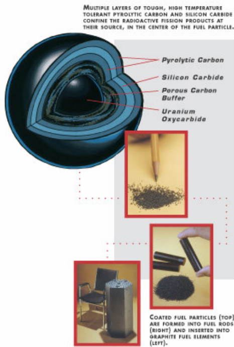
Figure 1-7: Prismatic fuel from 0.5 mm TRISO particles to the hexagonal fuel blocks (from [13])
