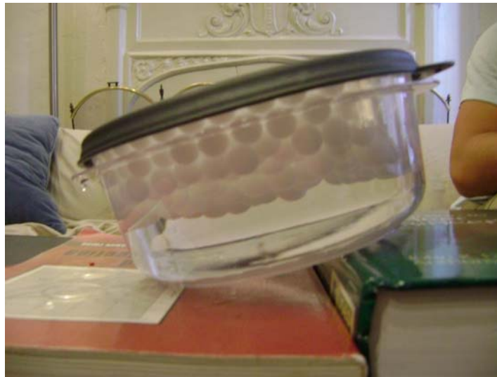
Fig. 5-20 The Static Angle of Repose experiment.
