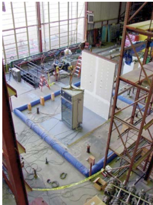
Fig. 5-11 View of the shake table at the Richmond Field Station (study investigating the seismic response of laboratory equipment). Courtesy of RFS.
