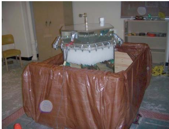
Fig. 5-18 Pebble Seismic Test Experimental System in Davis Hall.
