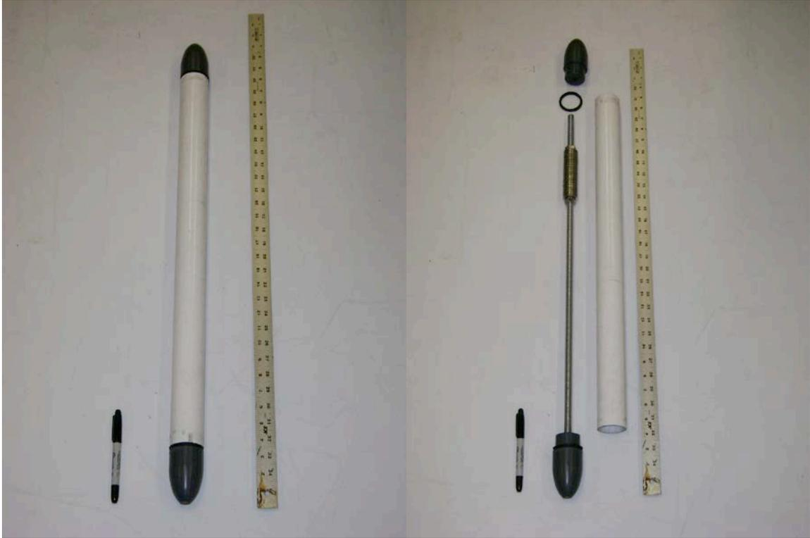
Figure 0-3 Pictures of the shutdown rod assembled and disassembled (yardstick provided for reference)
