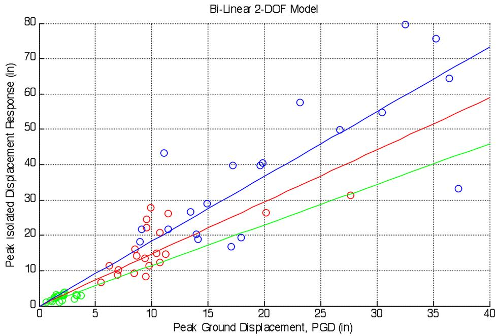
**Fig. 18** Peak displacement response of linear-elastic and bilinear isolator models with linear-elastic superstructures
