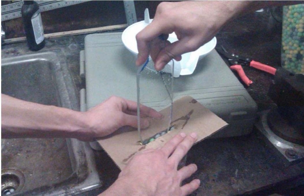
Figure 6.3: Insertion test of blunt end of blade into packed bed of spheres.
