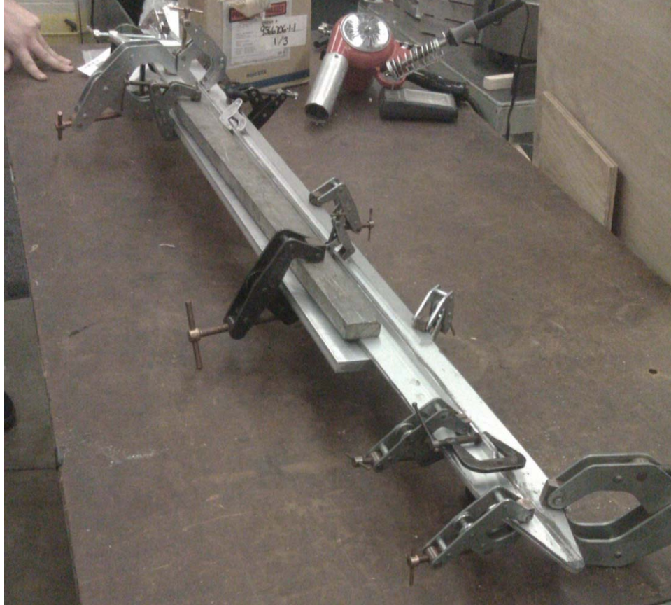
Figure 4.5: Experimental rod sections glued together with JB Weld
