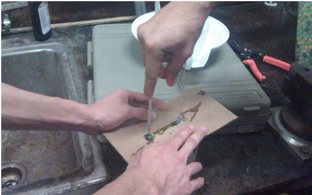
Figure 6.4: Insertion test of pointed end of blade into packed bed of spheres.
