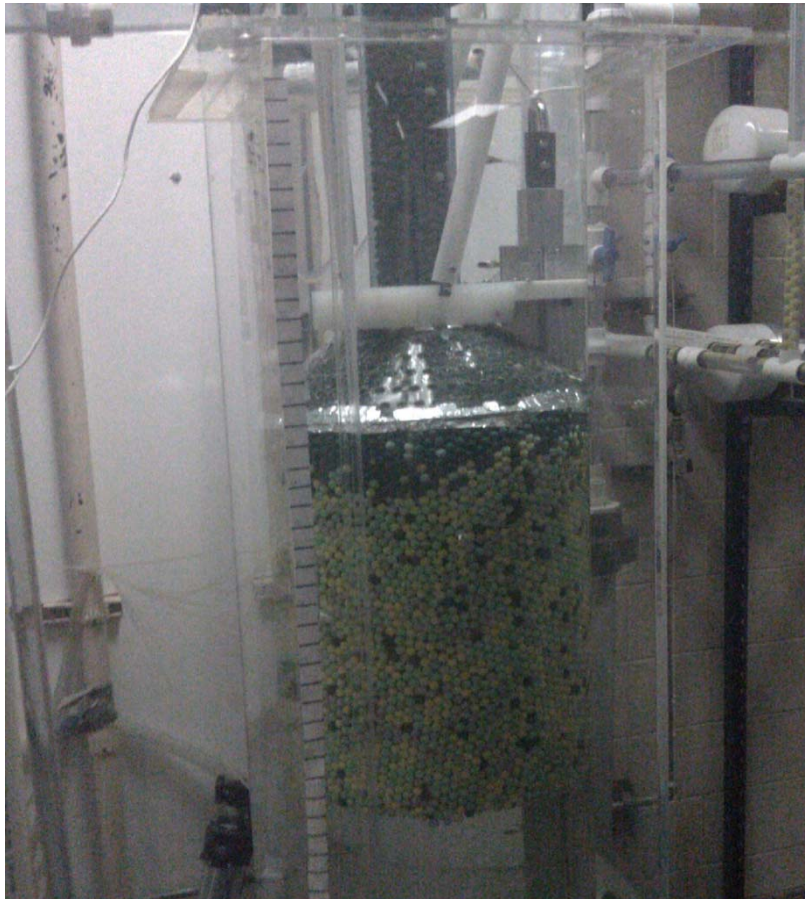
Figure 6.7: Full rod insertion into unpacked core.
