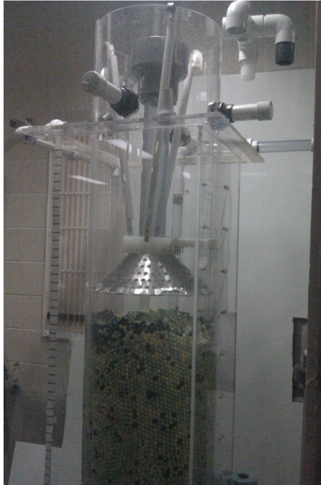
Figure 6.1: Retrofit of pebble recirculation experiment, PREX-1
