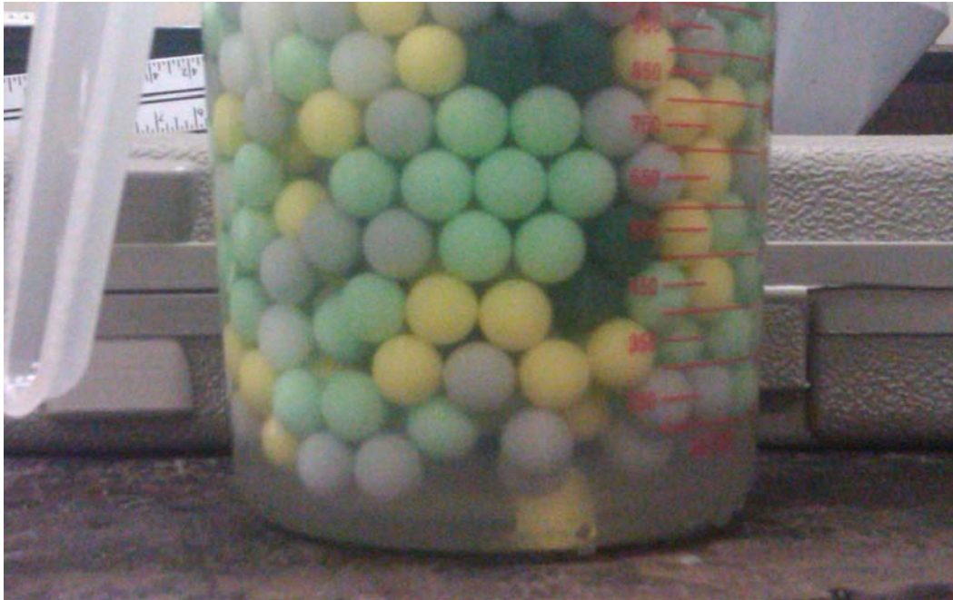
Figure 6.5: Blunt end tends to pin spheres during insertion which could cause rupture of fuel pebbles on impact.
