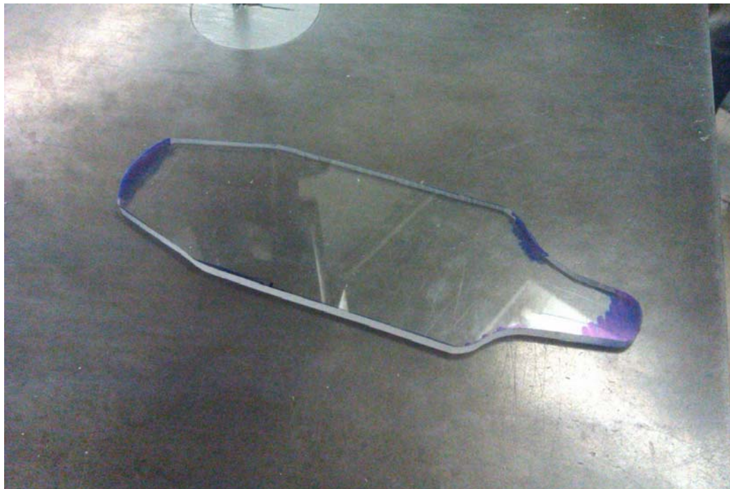
Figure 6.2: Test blade with blunt end on left and pointed end on right. The Blunt end should need greater force to insert due to the larger surface area causing higher friction forces, and the pointed end should need less force to insert due to smaller surface area.
