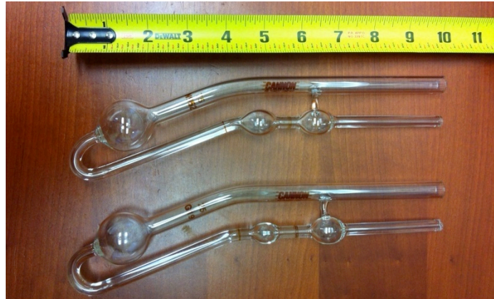
Figure 4-4. Cannon-Fenske glass capillary viscometers used for measuring oil kinematic viscosity.
