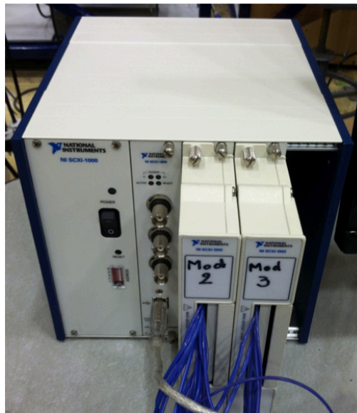
Figure 4-5. CIET 1.0 DAQ located at the operator workstation.
