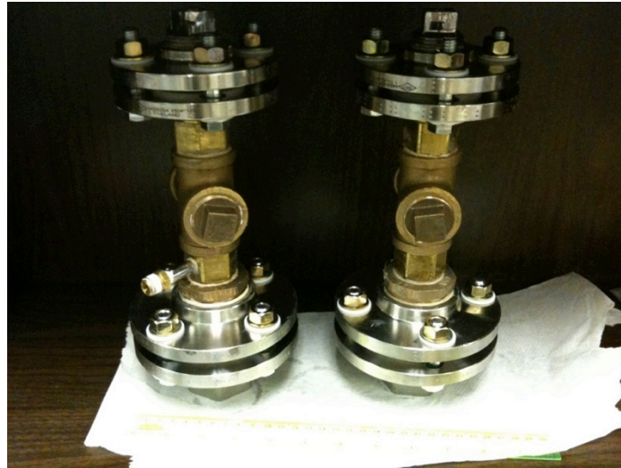
Figure 2-2. Assembled end-sections for the annular heater element tested on the CIET Test Bay. For complete assembly of the annular heater element, two concentric tubes slide into the end sections.
