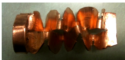
Figure 2-5. 2.5-cm-diameter, 4.3-cm-long flow mixer prototype.
