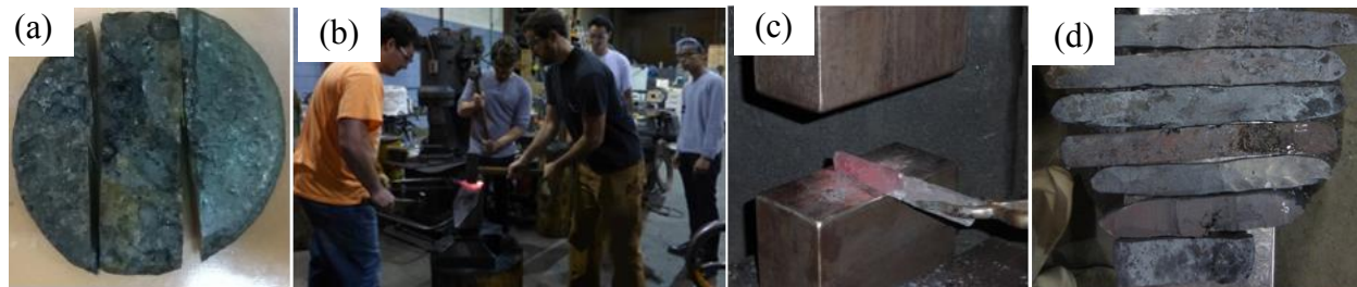
Figure 6: (a) A sponge iron ingot segmented into three strips; (b) and (c) hand forging the segments in (a) into thin strips; (d) resulting hand-forged strips from one session.
