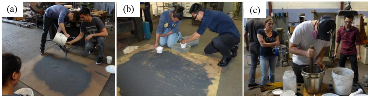
Figure 1: Filtering magnetite-enriched sand from the local northern California beach. (a) Spreading the sand on a cleaned flat surface; (b) carefully collecting magnetite from the sand with neodymium magnets in plastic cups; and (c) grinding the charcoal and mixing in the \text{CaCO}_3 for the smelting process.
