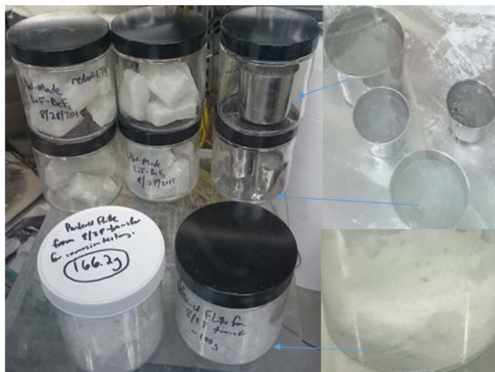
Figure 3.6: Total of 2.2 kg of UW-made FLiBe currently stored in glass jars. Four nickel crucibles are all fully filled with FLiBe. Approximately 250 g of granulated salt was separated for one crucible in corrosion test.
