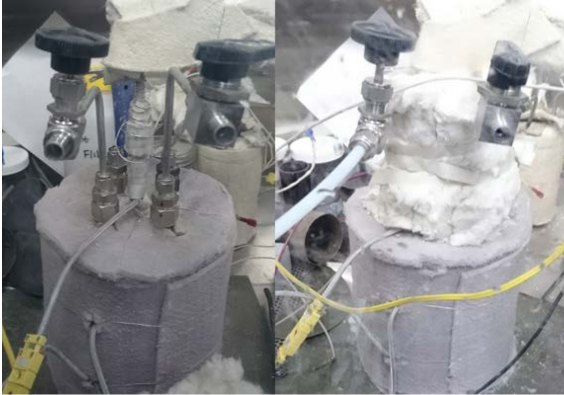
Figure 3.4: Nickel transfer vessel in glovebox (left) without insulation showing trace heating of transfer tube and (right) insulated with gas inlet to control pour rate secured.
