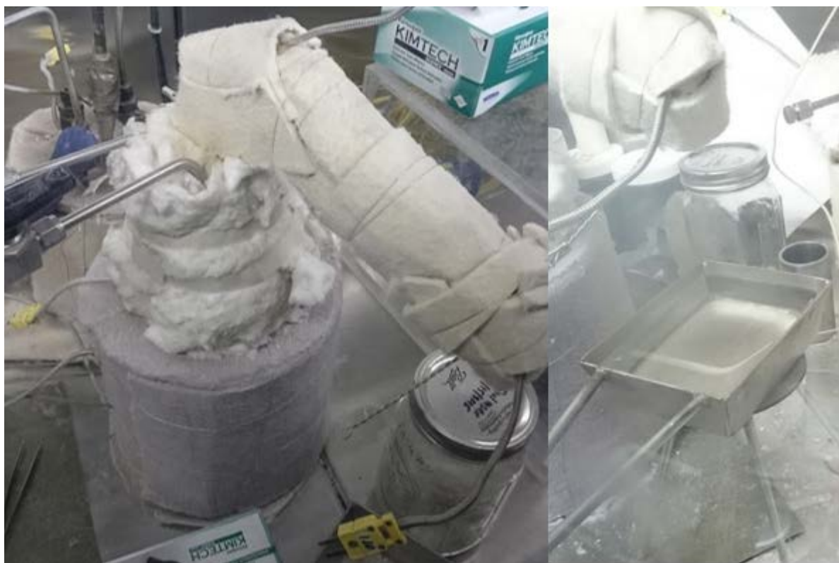
Figure 3.5: Complete transfer apparatus on left. Liquid FLiBe in Ni tray on right is completely translucent and flows fluidly. Provided adequate trace heating, salt can be poured by controlling Ar gas pressure through valves.
