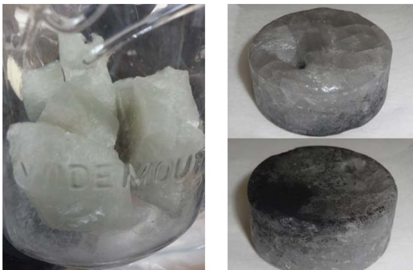
Figure 3.15: Initial MSRE FLiBe (left) and a salt ingot following an electro-purification run (right). The bottom of the ingot is facing upwards in the bottom right photo. The green tint in the initial salt is likely caused by dissolved metal fluorides. Reduction of these metals during plating also results in the dissolution of the carbon anode.
