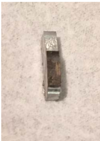
Figure 3.31: Photograph of in-reactor corrosion tested Hastelloy N, ~6.7mmx2mmx1mm, sectioned by using a low speed sectioning saw in MIT nuclear reactor laboratory. Sample was glued on aluminum strip for cutting.
