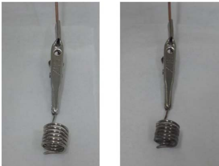
Figure 3.14: Nickel coil before (left) and after (right) electroplating. Plating results in a dark electrode surface likely from salt impurities.
