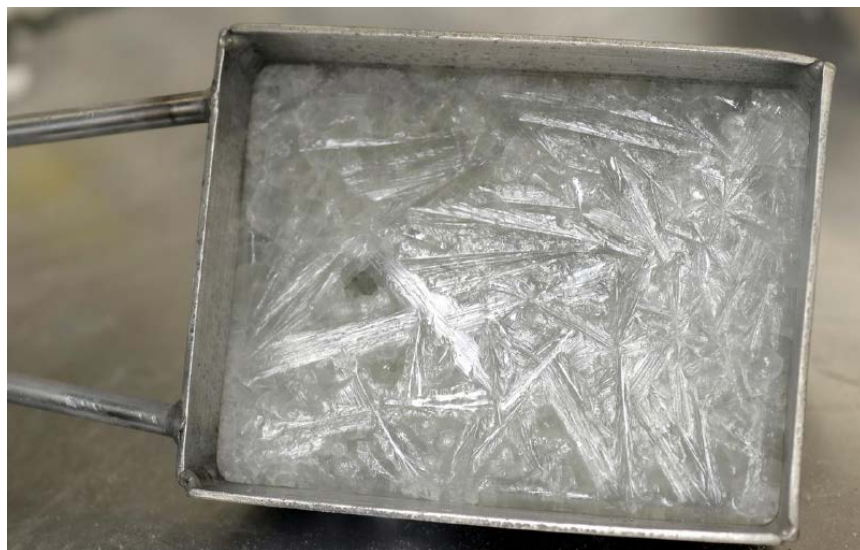
Figure 3.3: Purified FLiBe prepared from raw materials, lithium-fluoride and beryllium-fluoride.
