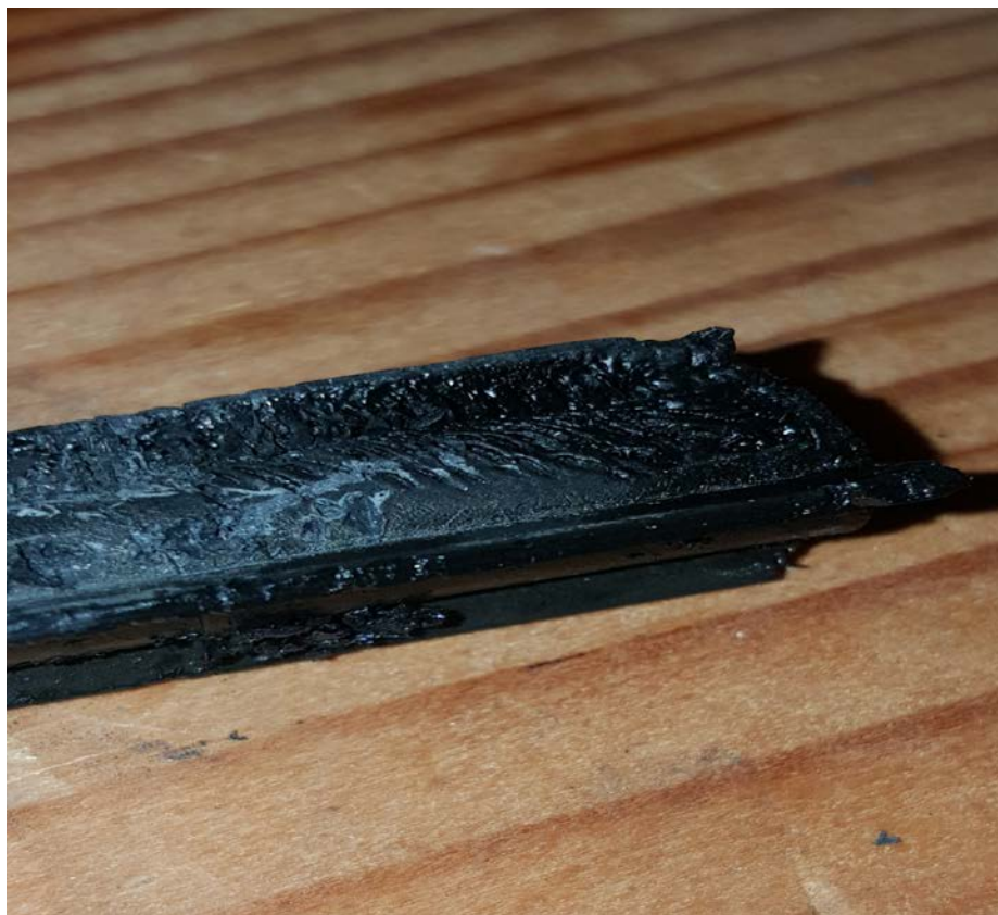
Figure 84. Close-up of material degradation from contact with medium-temperature oil.
