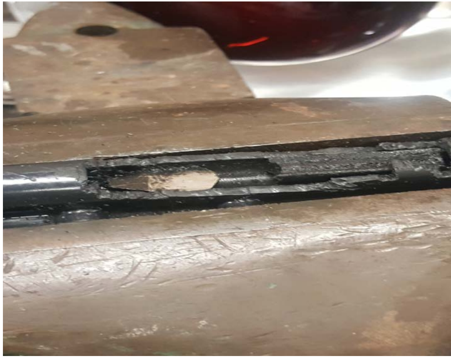
Figure 83. Heater outlet internals after degradation in contact with oil.
