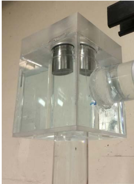
Figure 13: Flowing fluid study test section with no bubbles. It is possible to see how the flow must pass by the ultrasonic horn and how small the flow cross section is past the horn
