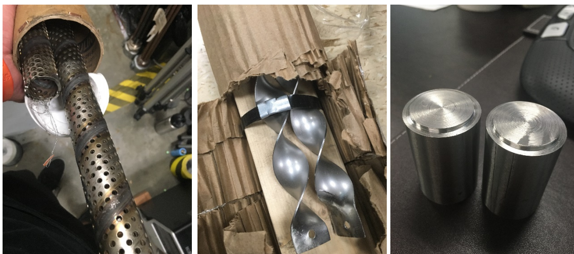
Figure 67. Components of the new inner assembly for the CIET heater: perforated tubes (left), twisted tapes (center), and end caps (right).
