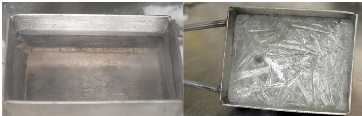
Fig. 6 Purified natural lithium FLiBe prepared from raw materials, lithium-fluoride and beryllium-fluoride: (a) the molten salt after extraction in inert atmosphere. (b) solidified FLiBe salt [3].
