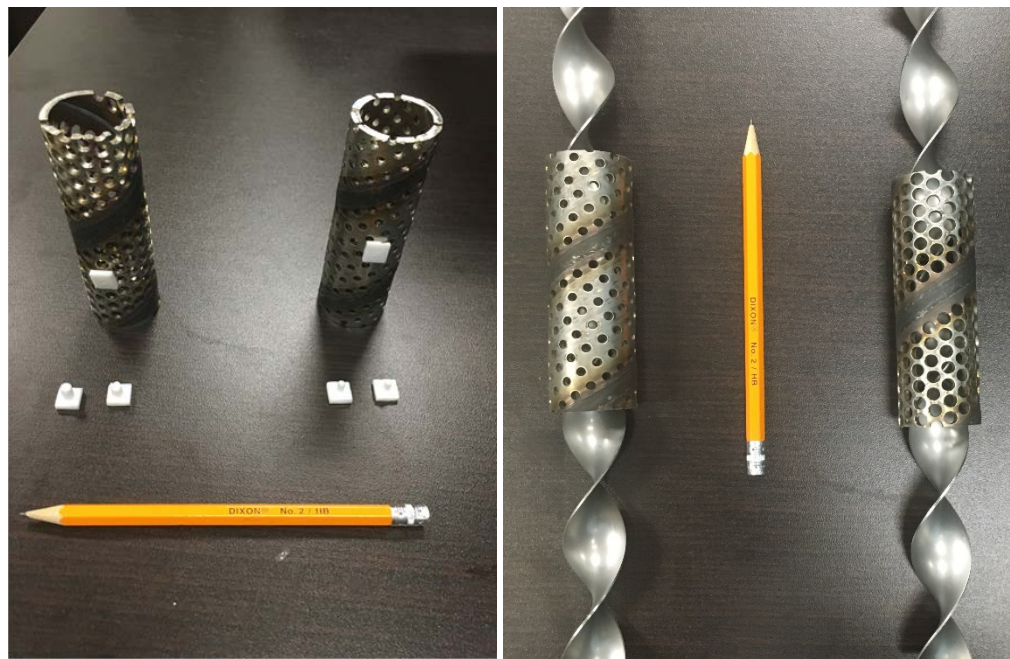
Figure 66. Detailed view of segments of the perforated tubes with the Teflon spacers (left) and twisted tapes (right); note the spiral weld seams.
