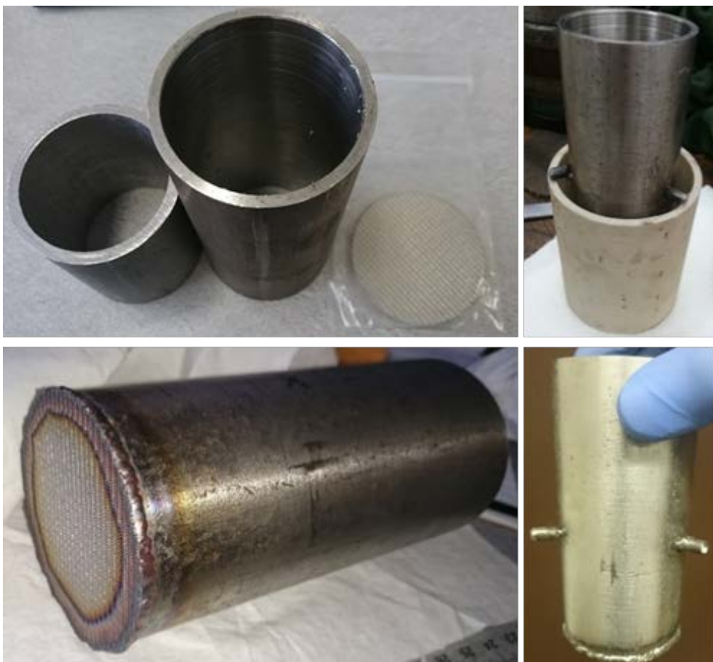
Fig. 8 Photographs of 316 stainless steel filter-bottomed crucible used for filtering metallic particulates generated from Be reduction [5].
