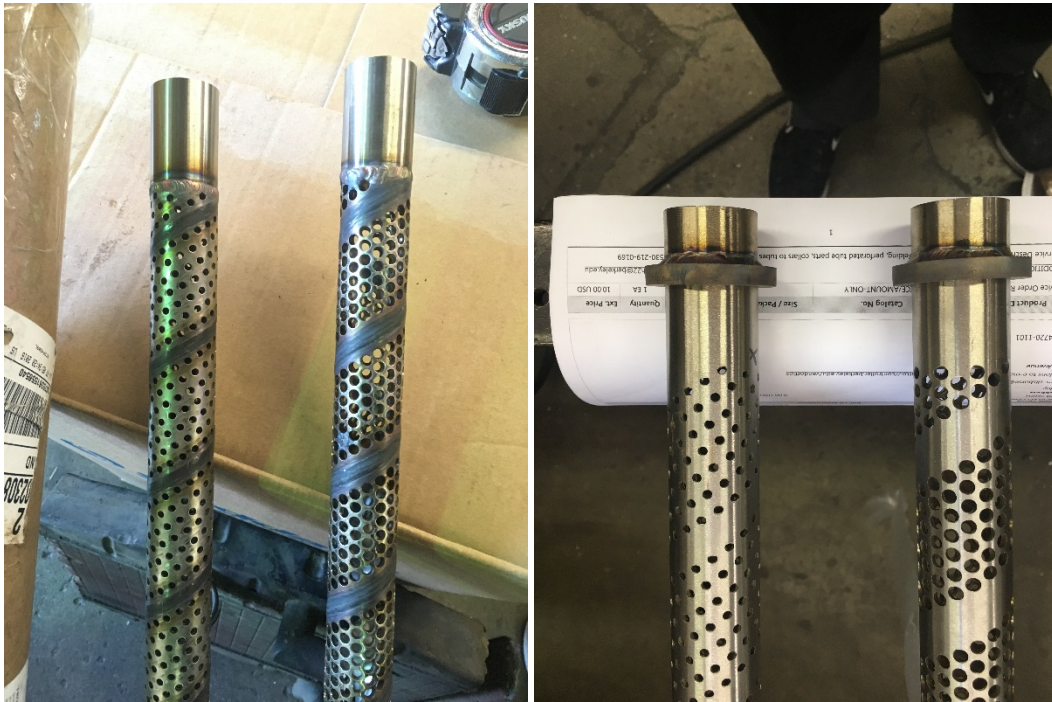
Figure 68. Finished heater assembly before centerless grinding and the addition of the support collar (left) and after (right).
