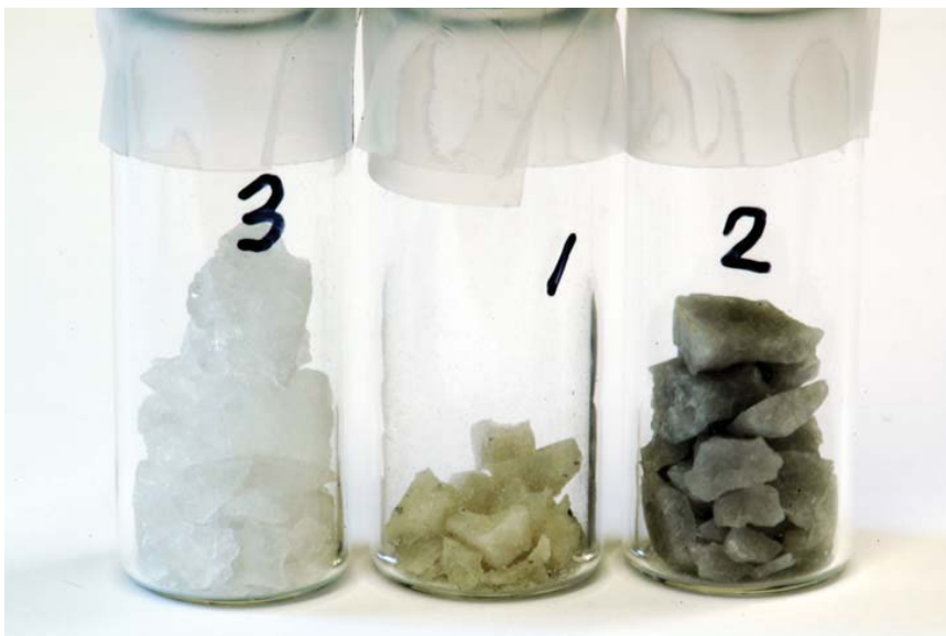
Fig. 4 A comparison of University of Wisconsin FLiBe and MSRE FLiBe. From left to right: re-purified MSRE FLiBe, salt melted in open atmosphere from raw components, salt melted in a glove box from raw components [3].
