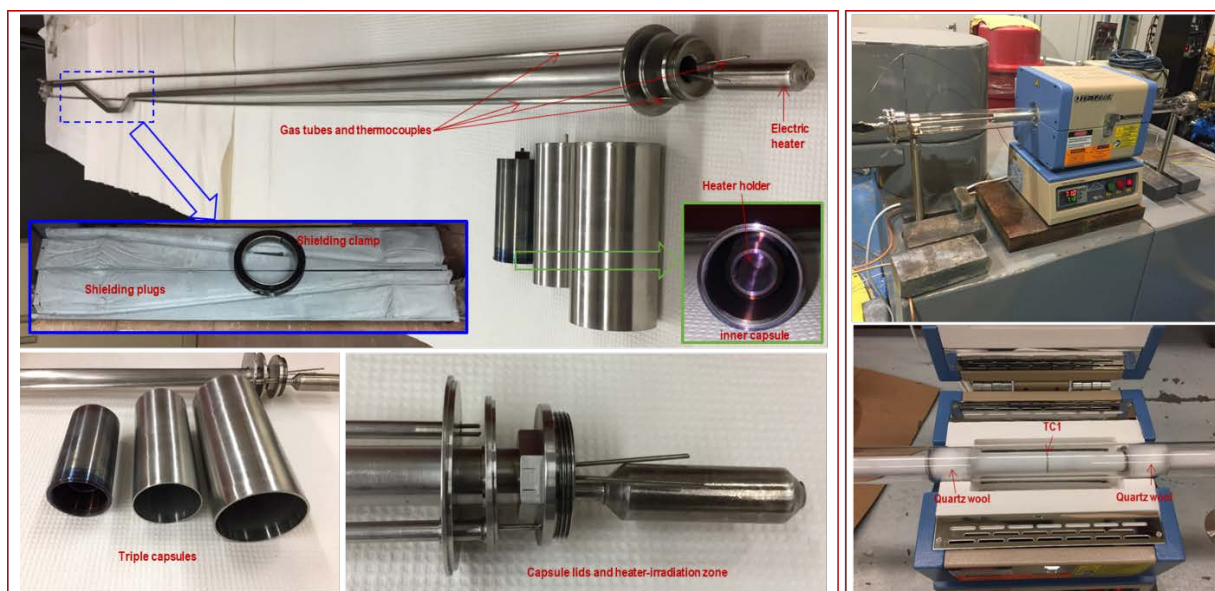
Figure 11: (left) main components for salt neutron irradiation and (right) high-temperature tube furnace.
