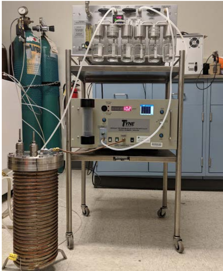
Figure 2. Thermal desorption measurement setup with the furnace, ion chamber, and tritium bubbler in the experimental configuration.
